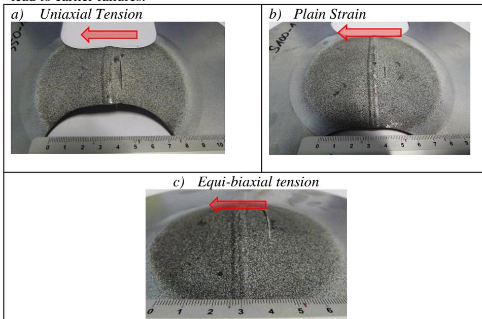
Fig. 3 – Movement of the weld line.
