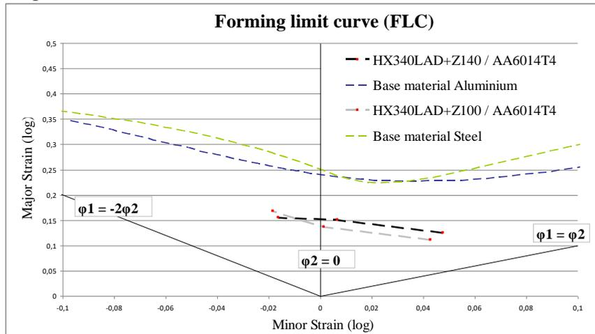
Fig. 5 – Forming limit curve for THB.
