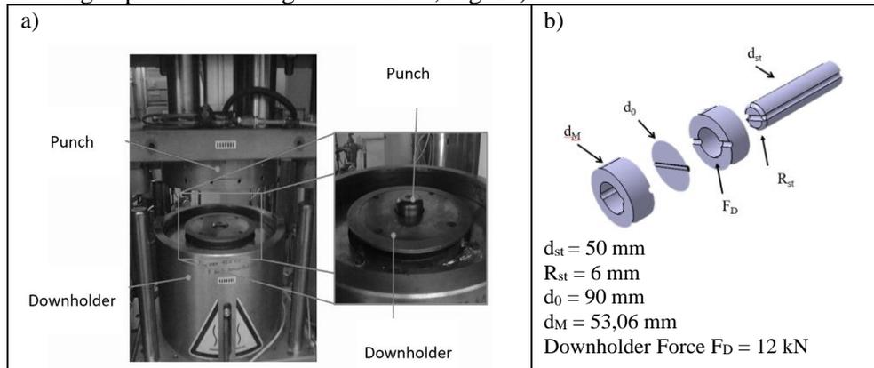
Fig. 2 – Cup Test Equipment.
