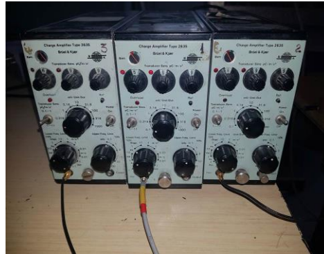
Fig. 9 – Bruel&amp;Kaer Charge Amplifiers Type 2635.
