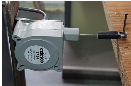
Fig. 6 – Celesco SP2-4 displacements sensor.
