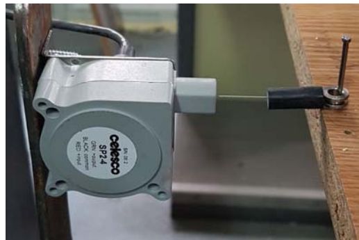
Fig. 6 – Celesco SP2-4 displacements sensor.
