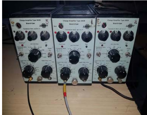
Fig. 9 – Bruel&Kaer Charge Amplifiers Type 2635.
