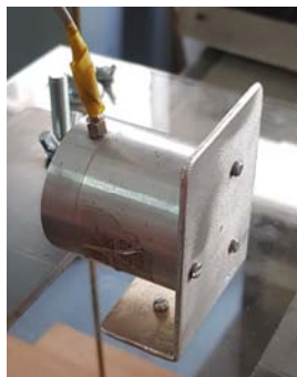
Fig. 7 – Charge Accelerometer HMF KB12.
