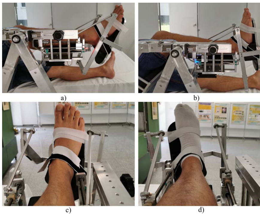
Fig. 10 – Screenshot of RECOVER parallel robot for ankle rehabilitation during the test: a) plantar flexion; b) ankle dorsiflexion; c) ankle eversion; d) ankle inversion.
