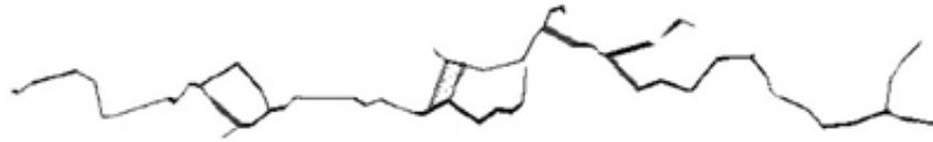
Fig. 6 – Stress corrosion morphology of crack pattern.
