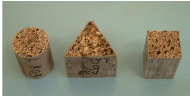
Fig. 1 – Different shapes of AAFs for compression tests (AlMg1Si0.6 + 1% wt. ZrH 2 , height 30 mm).
