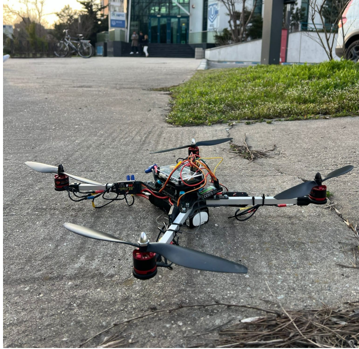
Fig. 4 – Photograph of the actual quadcopter test platform equipped with the developed controller
